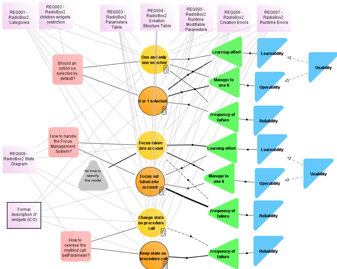
Figure 8. Snapshot of the DREAM diagram for the design of the behavior of the ARINC 661 RadioBox2 widget
